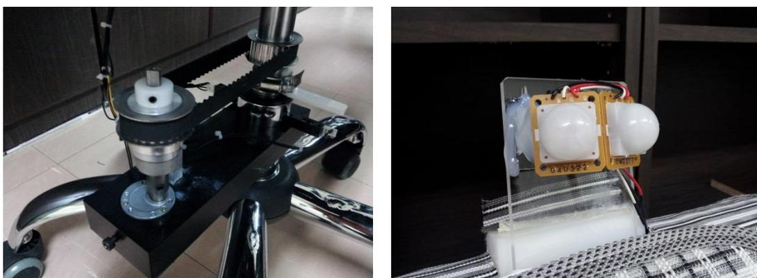
Figure 7. Rotation clutch & sensor controller and detecting a human body Sensor
