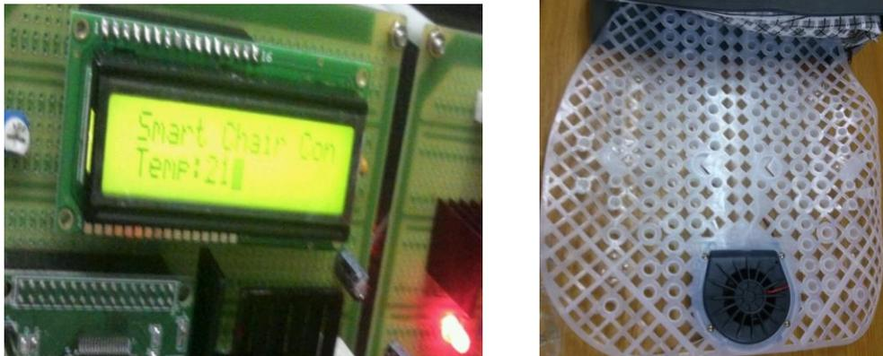
Figure 9. Temperature checked with LCD and fan additionally mounted at the seat
