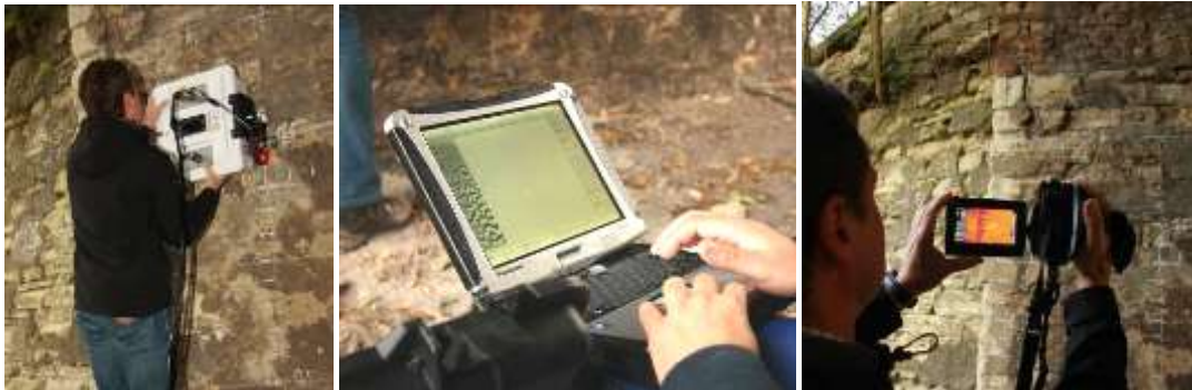
Figure 3. GPR and infrared thermography testing on stone arch bridges.
