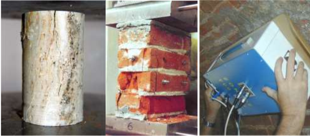
Figure 1. Examples for laboratory and in-situ diagnostic procedures. From left to right: compression strength test of a stone core sample, compression strength test of bricks, radar survey on an arch.
