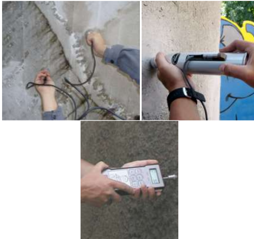
Figure 5. Site tests on real rehabilitation projects. From left to right: ultrasound test, Schmidt-hammer hardness test, penetration.
