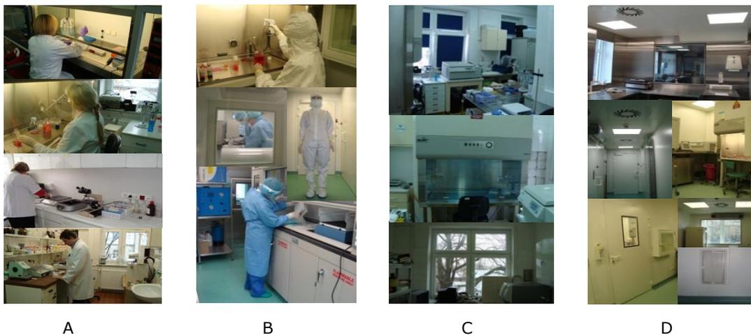
Figure 2. A. Every-day work and reality in university labs; B. Working in clean rooms; C. Interiors of regular labs at the university; D Interiors of clean-rooms, specific design elements – glassed doors, internal windows, windows for material flow, ventilation system, special material for wall and floor surfaces, merging of floor and wall surface.
