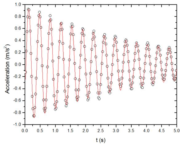
Figure 7. Experimental acceleration data (open circles) and fitted curve (solid line) for the damped harmonic motion.
