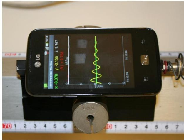
Figure 6. A close-up of the smartphone moving with damped oscillations.
