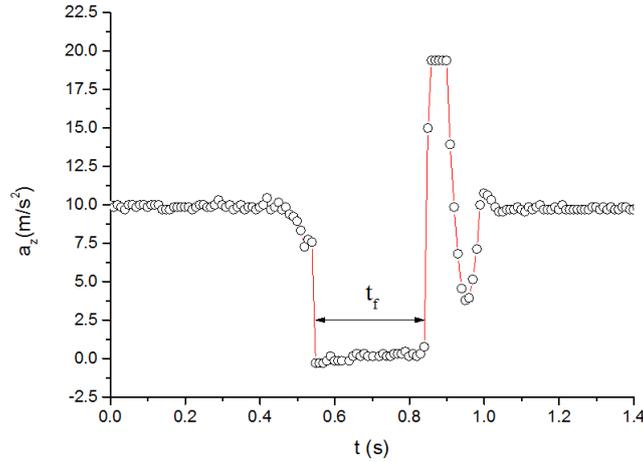
Figure 2. Acceleration sensor measurements for the free fall time of the smartphone.
