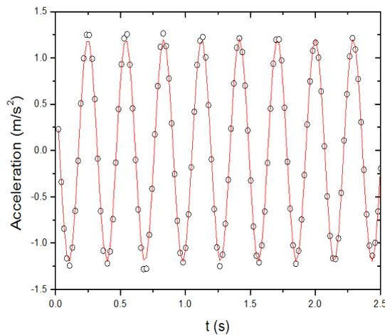
Figure 5. Experimental acceleration data (open circles) and fitted curve (solid line) for the free harmonic oscillation.
