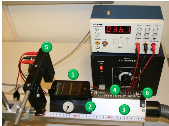
Figure 4. Photograph of the experimental setup with the smartphone moving with free oscillations.
