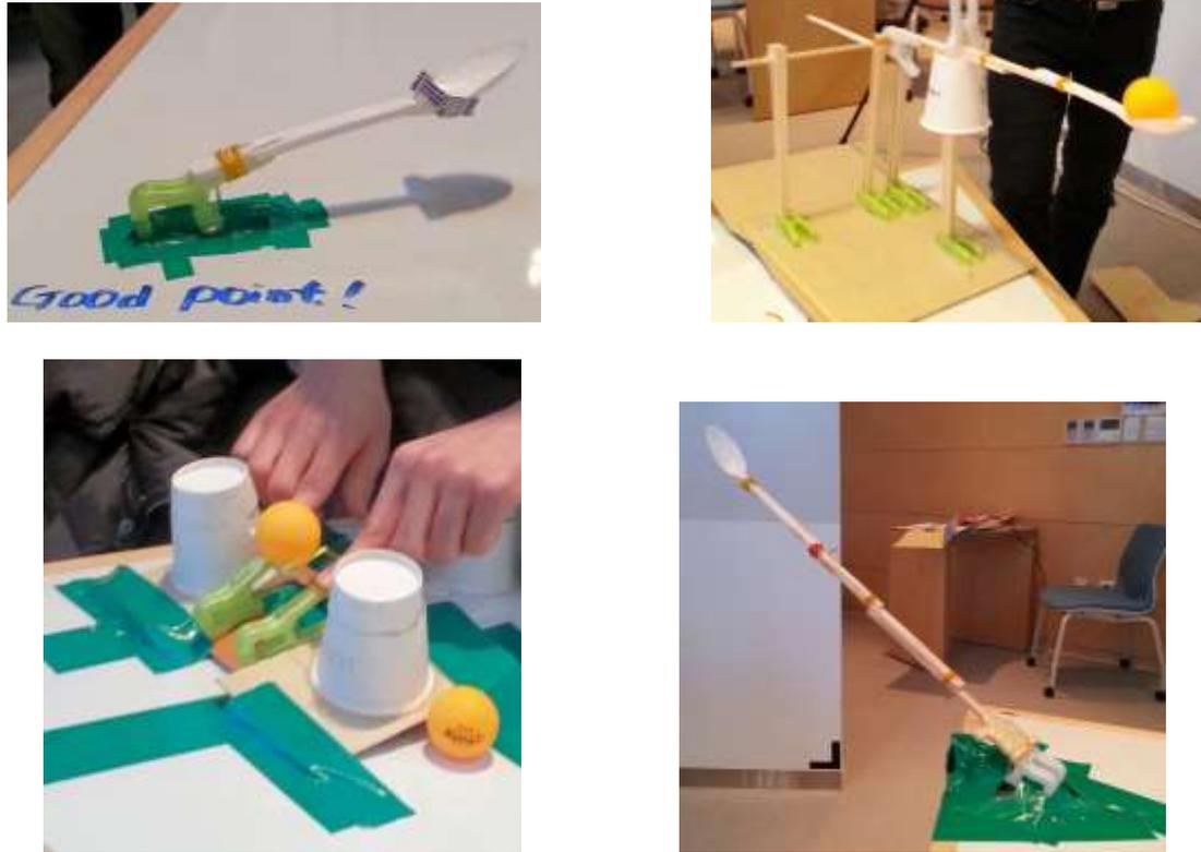
Figure 3. Examples of prototypes designed toward the testing phase of the design, with plenty of time given for alternative designs and testing. Precision was set at 30 cm. The target was a trash can, and the ping-pong balls (orange color) were used with the designed catapults. See text for details.
