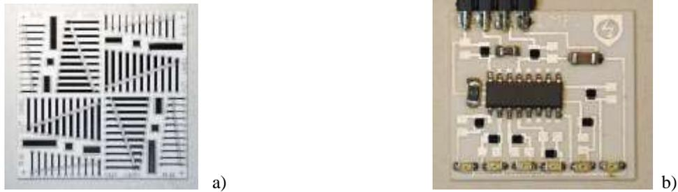
Figure 5. Examples of HIC's realized in lab a) passive resistor network b) functional HIC.
