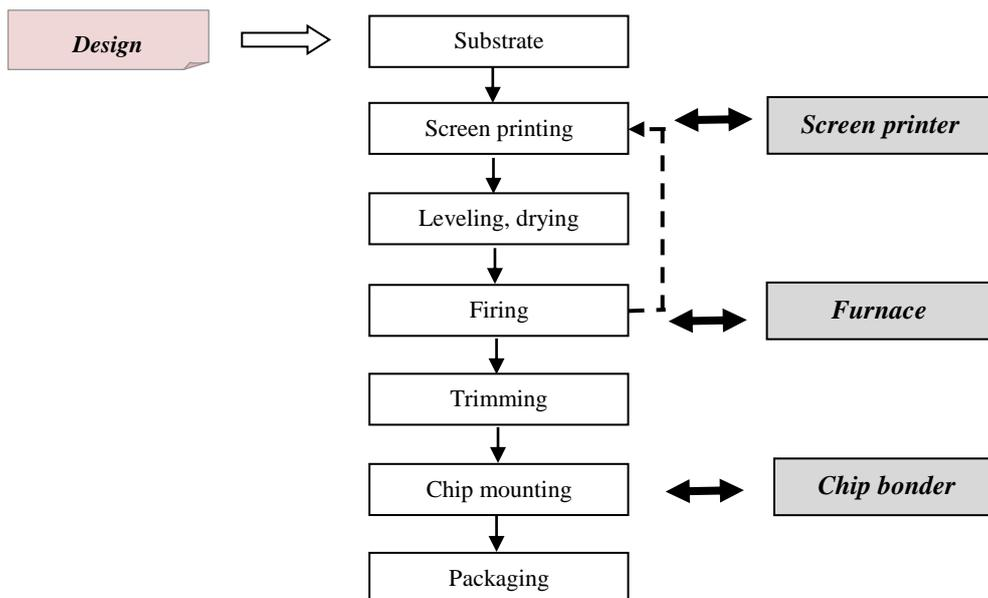
Figure 2. Technology process for realization of HIC.
