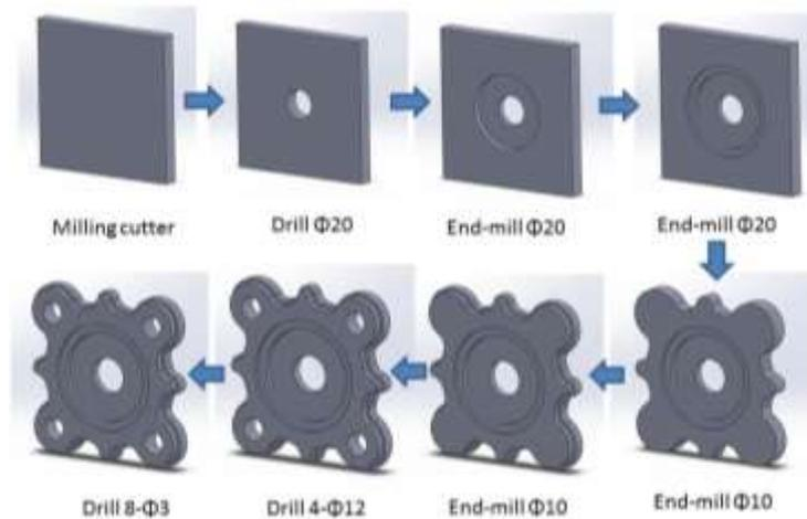
Figure 31. Sequence of machining.
