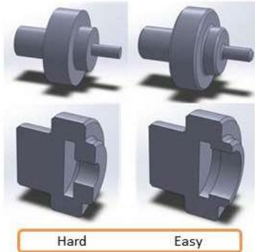
Figure 13. Lathe machining
