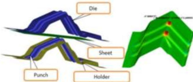
Figure 18. Forming simulation.
