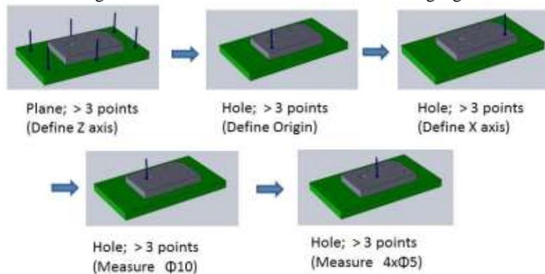
Figure 33. Measuring process using 3D coordinate system
