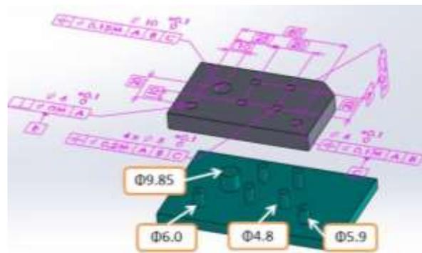
Figure 32. 3D-annotated model and functional gauge.
